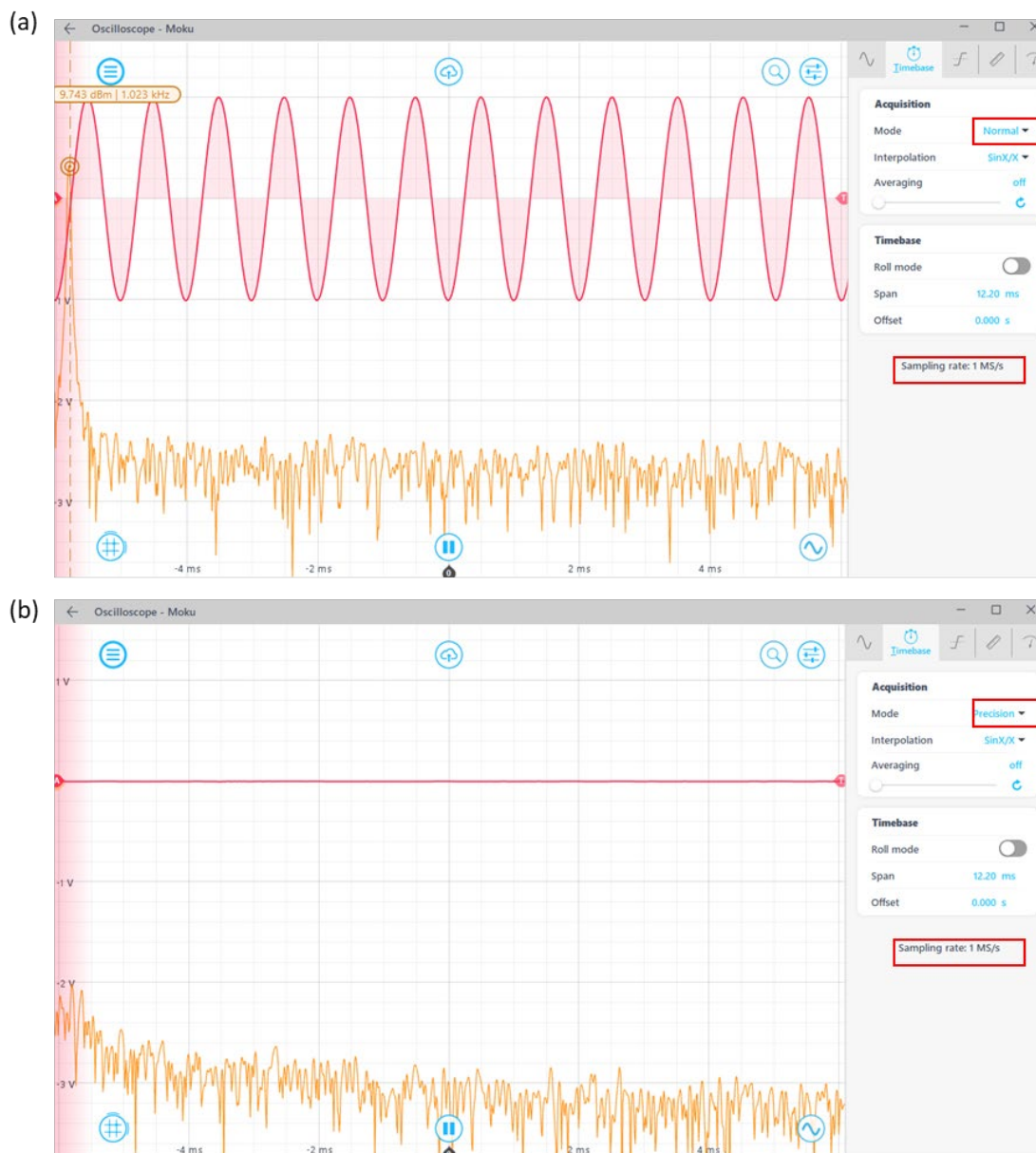
Figure 5: A 2.001 MHz signal was captured with the averaging disabled (a) and enabled (b). The aliasing effect was significantly reduced with the precision mode enabled.
