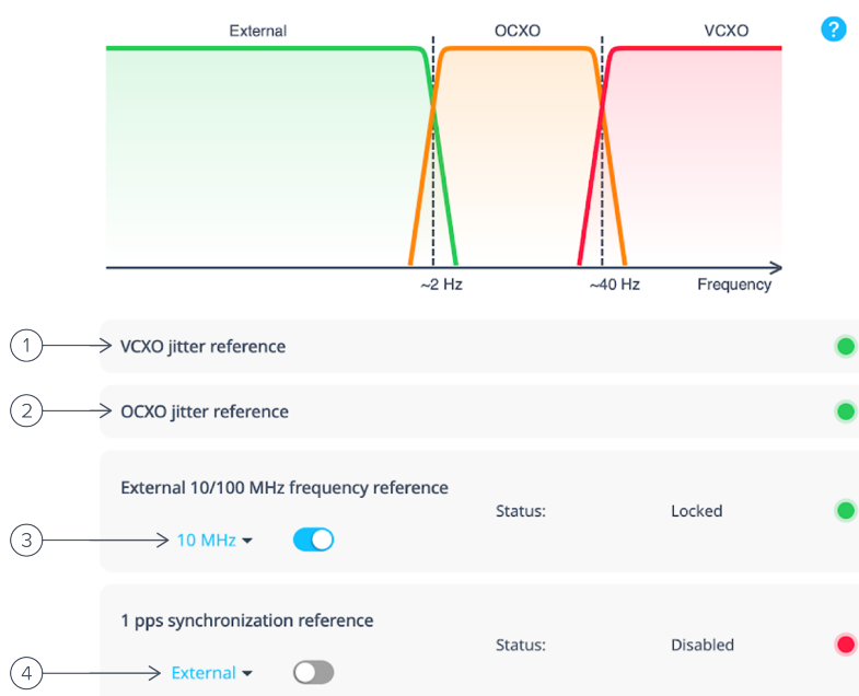
Figure 23. Moku clock blending configuration dialog with an external 10 MHz frequency reference enabled.
