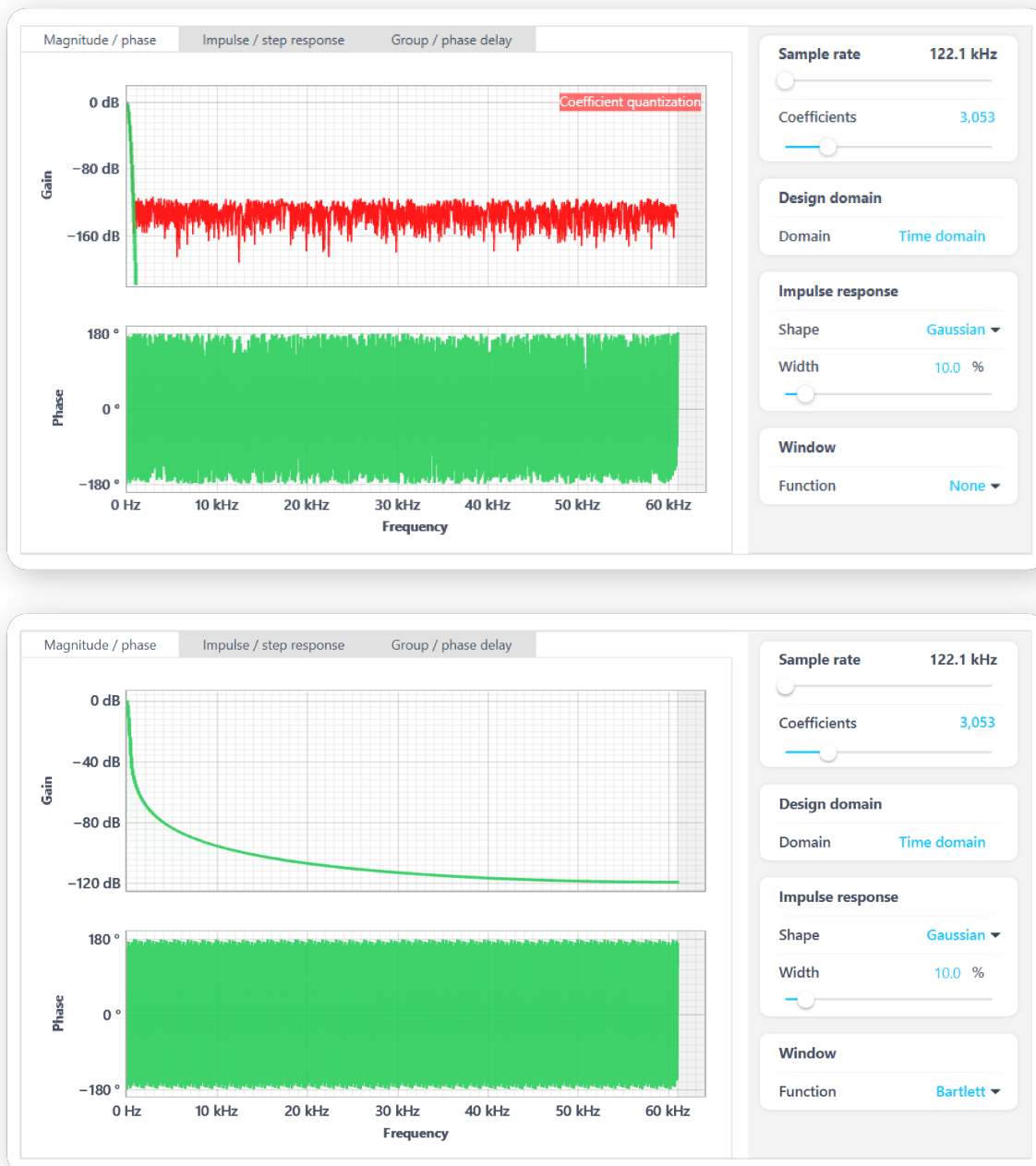
Figure 6. A 25 ms Gaussian FIR filter designed with 10 % width, 3,053 coefficients, 122.1 kHz sample rate, and a Bartlett window (bottom) to reduce the dynamic range, eliminating quantization artifacts evident in the unwound design (top).
