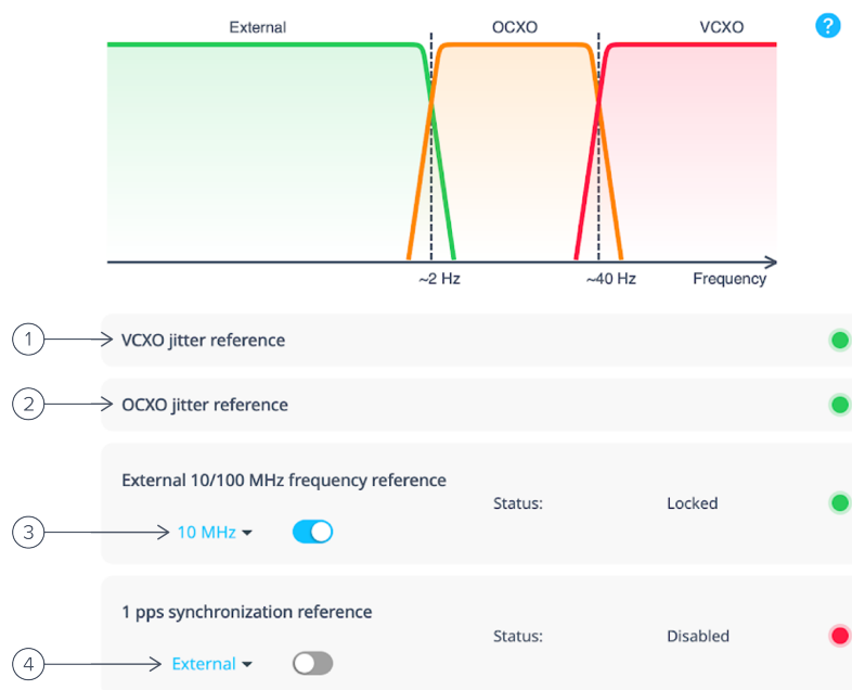
Figure 20. Moku clock blending configuration dialog with an external 10 MHz frequency reference enabled.
