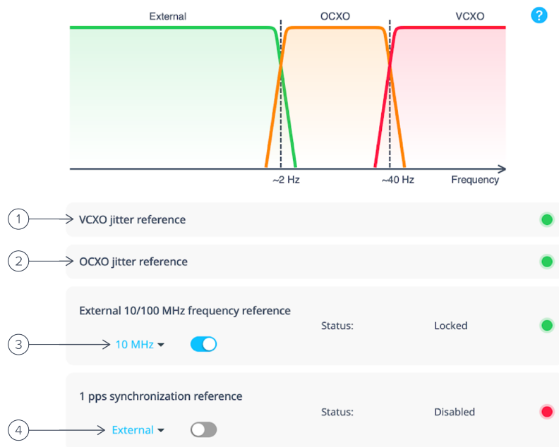
Figure 38. Moku clock blending configuration dialog with an external 10 MHz frequency reference enabled.
