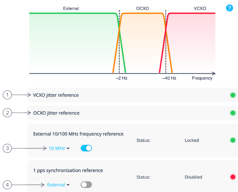
Figure 33. Moku clock blending configuration dialog with an external 10 MHz frequency reference and GNSS enabled.
