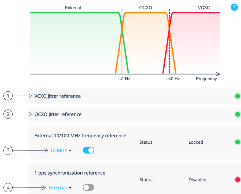
Figure 35. Moku clock blending configuration dialog with an external 10 MHz frequency reference and GNSS enabled.
