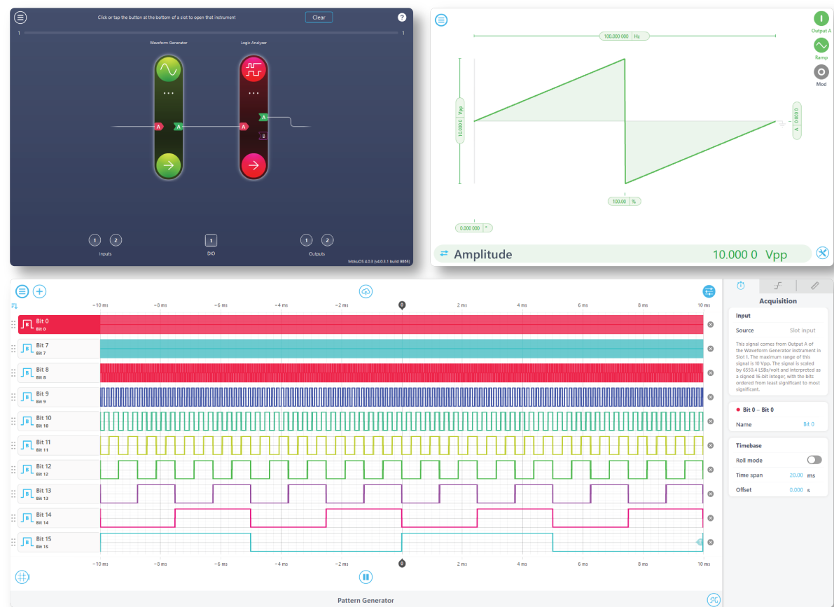
Figure 10. Routing analog signals to the Slot Input of the Logic Analyzer
