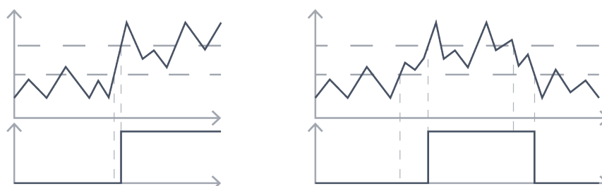
Figure 7. High/low thresholding analog to digital examples
