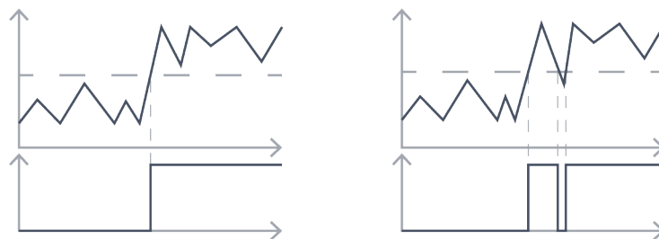
Figure 6. Single thresholding analog to digital examples
