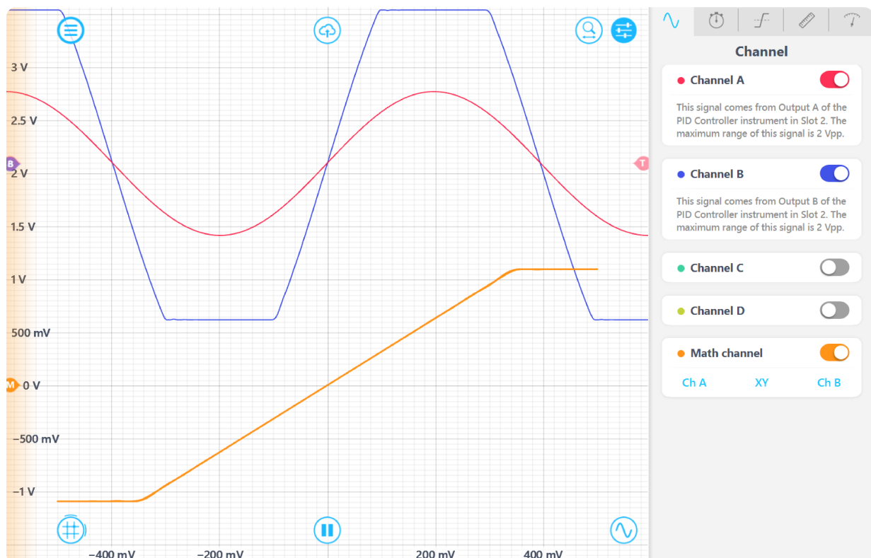
Figure 32. Op-amp input signal (Channel A), output signal (Channel B) and transfer curve (Math channel).
