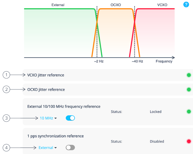
Figure 23. Moku clock blending configuration dialog with an external 10 MHz frequency reference and GNSS enabled.
