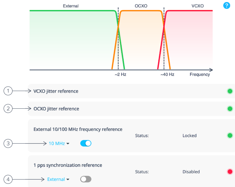
Figure 24. Moku clock blending configuration dialog with an external 10 MHz frequency reference and GNSS enabled.
