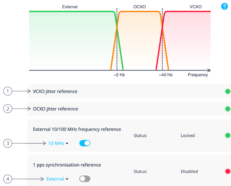
Figure 36. Moku clock blending configuration dialog with an external 10 MHz frequency reference and GNSS enabled.
