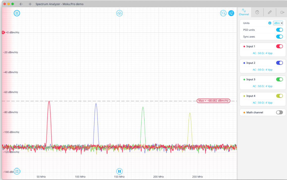
Figure 8. Spectrum Analyzer with dBm PSD units (dBm/Hz)
