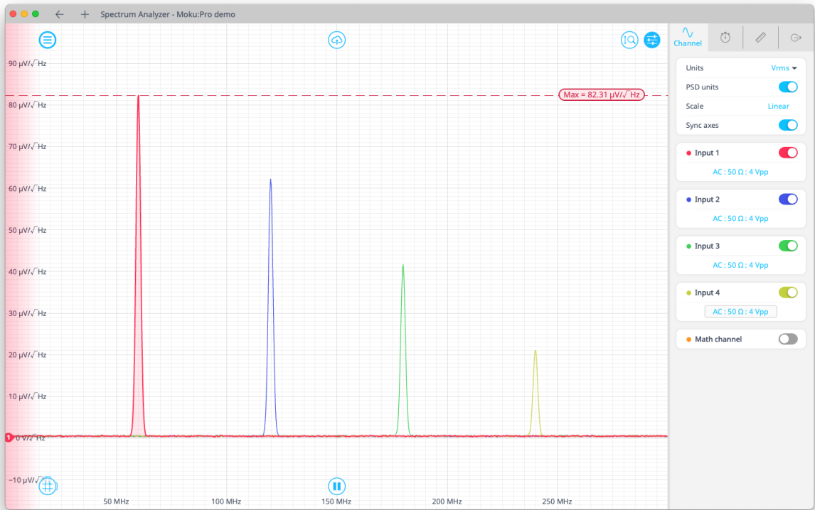
Figure 9. Spectrum Analyzer with Vrms PSD units ( \mu\text{V}/\sqrt{\text{Hz}} )
