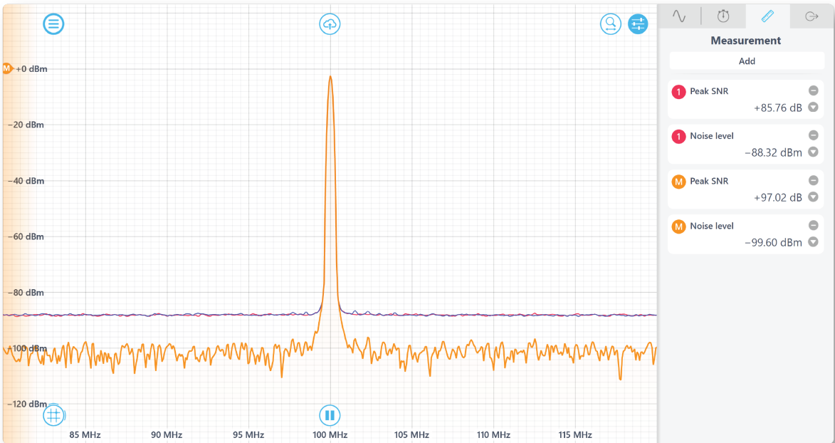
Figure 6. Noise floor and SNR measurements (right) of the cross-correlation channel.
