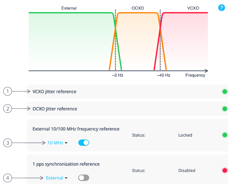
Figure 45. Moku clock blending configuration dialog with an external 10 MHz frequency reference enabled.
