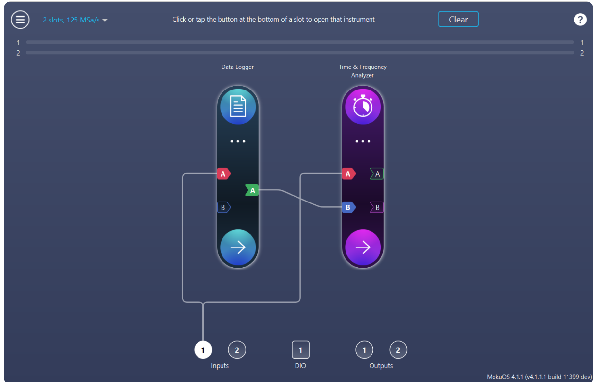
Figure 34. Multi-Instrument Mode, with Data Logger in Slot 1 and Time & Frequency Analyzer in Slot 2.
