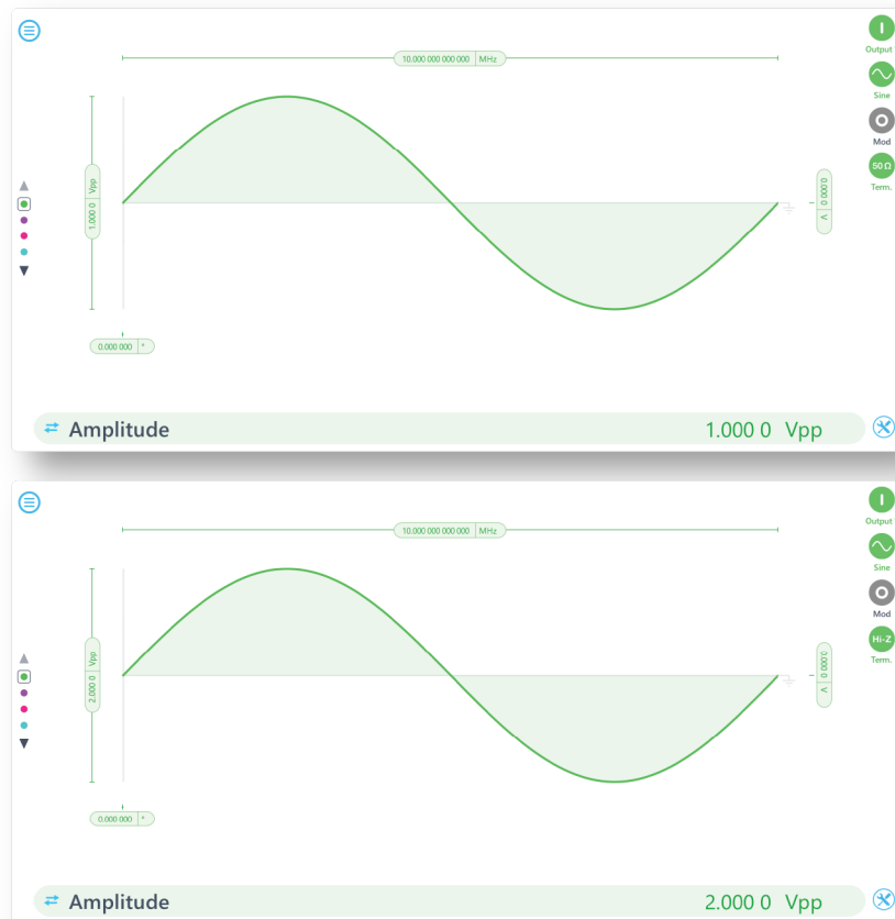
Figure 5. Relationship between termination and displayed amplitude
