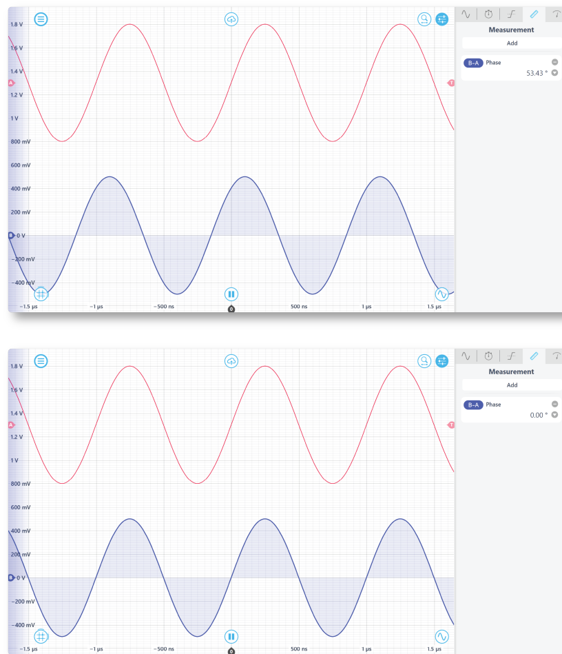
Figure 4. Sync waveforms in the Waveform Generator
