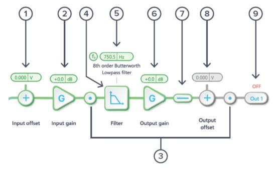
The two independent, real-time configurable digital IIR filter paths follow the control matrix in the block diagram, represented in green and purple for filters 1 and 2, respectively.
