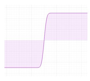
Gaussian interpolation smooths the signal out, preserving the visual characteristics of the signal at the expense of frequency information.
