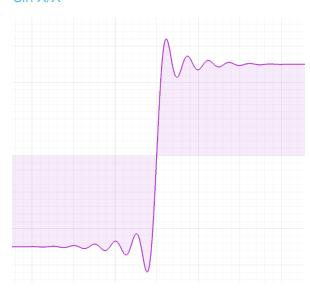
Also called "Sinc" interpolation, this mode preserves the frequency characteristics of the signal. In the time domain, it can appear that there is over- or under-shoot that is not present in the signal.
