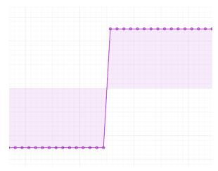
Linear interpolation does not perform any up-sampling. On the display, it marks each point in the original data set and draws a straight line between them. This display does not invent any new data points.
