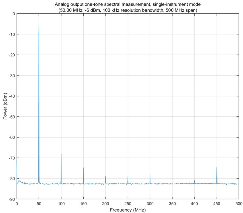
One-tone spectral measurement 50 MHz, -6 dBm (100 kHz RBW, 2.5 GHz span)
